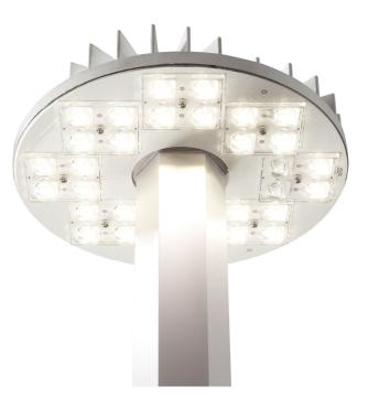
The P4 is our fourth generation flat array with 30 LED emitters and was designed to increase roadway performance while providing superior spacing. Utilizing a refractor optic, the P4 is perfect for roadway applications requiring a uniform footprint.
