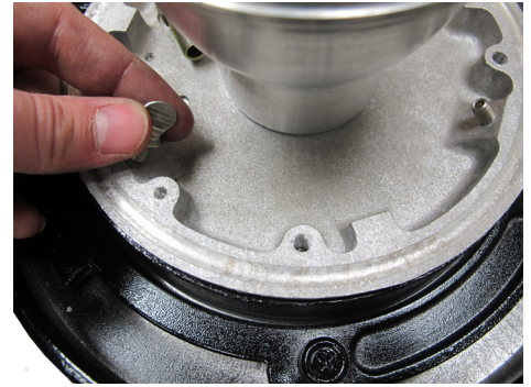
STEP 3: REMOVE THE BALLAST PLATE AND ASSEMBLY FROM THE HID FIXTURE
